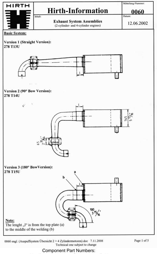
Manifold: 278A1U Silencer: 278E4U Diffuser Cones: 278T19U (Straight), 278T20U (90deg), 278T21U (180deg) Manifold to diffuser Connectors: 278E19U (90deg), F308A7U (Straight) Distance (L) (See above) for all configurations = 30mm
